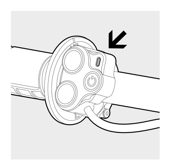
The control switch contains a **LED light** which can change color. Each color has a different meaning.
