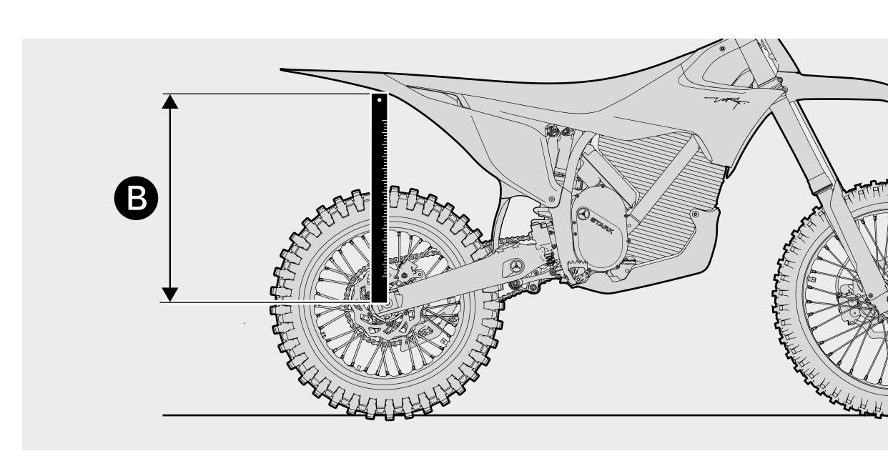
2 Place the bike with both wheels on the ground and measure the height B between the wheel axle and the SAG marking on the rear spoiler. Recommended value is: height A (see step 1) minus 40 mm to 45 mm.
