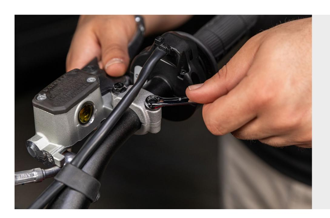
13 If your bike is equipped with rear hand brake instead of rear foot brake, repeat the previous step to attach the rear hand brake on the left side of the handlebar.
