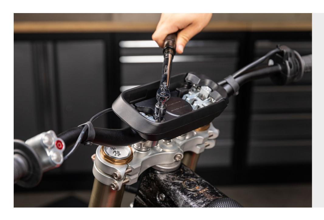
11 Tighten the four bolts inside the docking station to 30 Nm.
