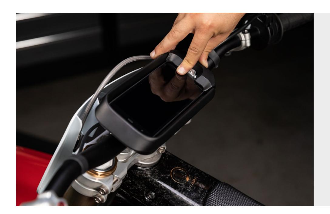
2 Connect the **Stark Future phone** with the supplied **charging cable** to a suitable power adapter and outlet.
