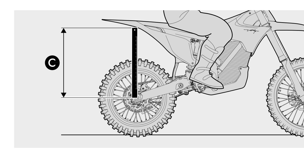
3 Place the bike with both wheels on the ground and, with a rider sitting on the bike, measure the height C between the wheel axle and the SAG marking on the rear spoiler. Recommended value is: height A (see step 1) minus 102 mm to 108 mm.
