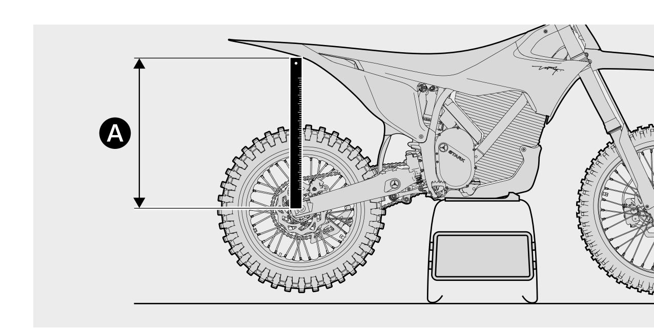
1 Measure the height A between the wheel axle and the SAG marking on the rear spoiler with the bike on the stand and both wheels off the ground.
